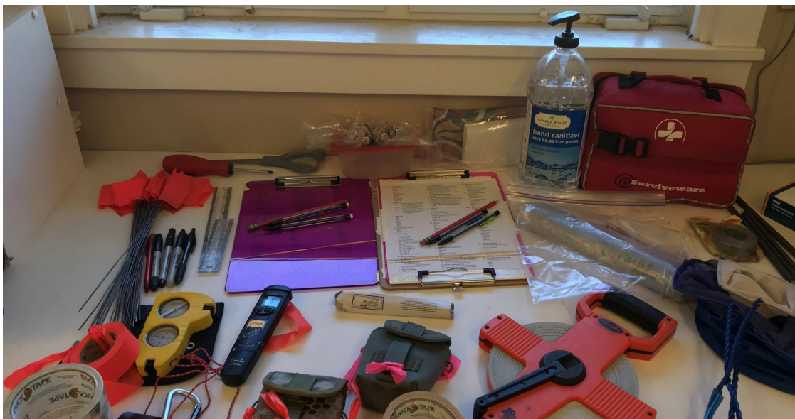
Fig. 11. Much of the basic equipment needed for a Level 2 springs inventory is shown in this photo. Necessary gear that is not shown in this photo includes the Solar Pathfinder, binoculars, equipment for measuring flow, a trowel or digging knife for harvesting plant specimens, a plant press, and vials and envelopes for preserving invertebrate specimens.
