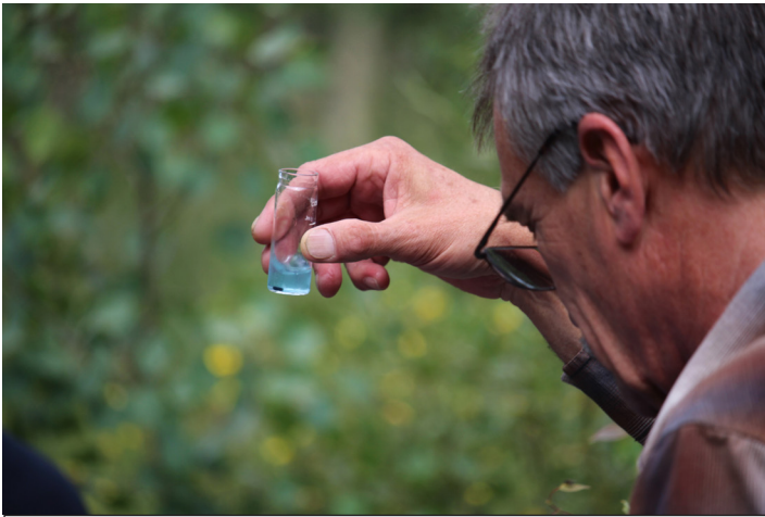
Fig. 51. Field test kits are available to measure water quality parameters, such as pH, alkalinity, and dissolved oxygen. These require no calibration, are relatively inexpensive, and provide a useful backup system for electronic units.
