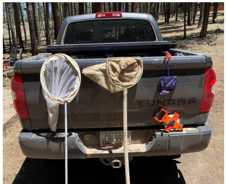
Fig. 22. Several types of nets used to collect invertebrates. The white aerial net (left) is used to collect terrestrial insects; the tan-colored D-net (middle) is used for aquatic invertebrate sampling in lentic or lotic habitats; and the small blue aquarium net is useful for sampling aquatic invertebrates in variety of habitats including small shallow streams.
