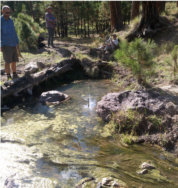
Fig. 49. At Horse Camp Spring in the Gila Wilderness, subaqueous flow emerged into a flowing springbrook, making discharge measurements impossible for a Level 2 survey.
