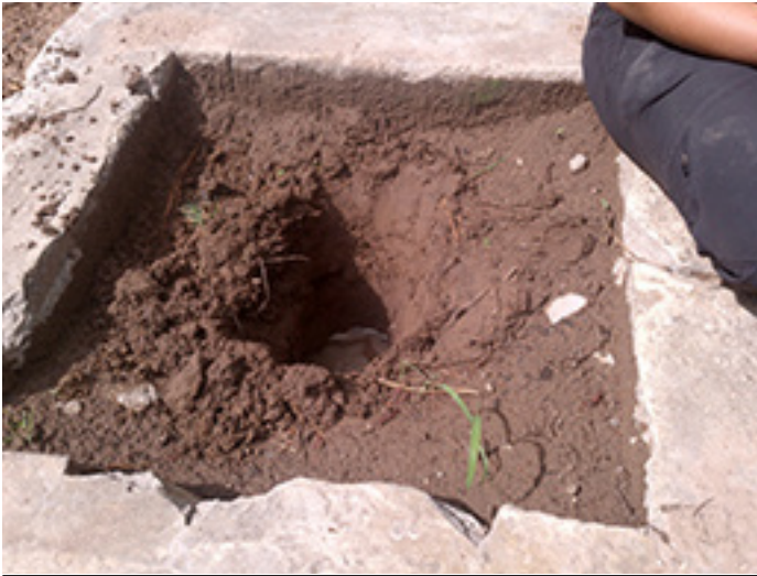
Fig. 48. This image shows the depression/sump flow estimation technique. In this case, surveyors dug a hole at the source and measured time to refill.
