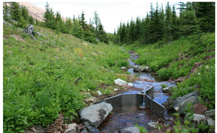
Fig. 45. A cutthroat flume is useful in low-gradient, relatively fine-grained channels. Although "portable", it is heavy and awkward for use in remote sites. This flume was used to measure flow at a rheocrene spring in Canada.
