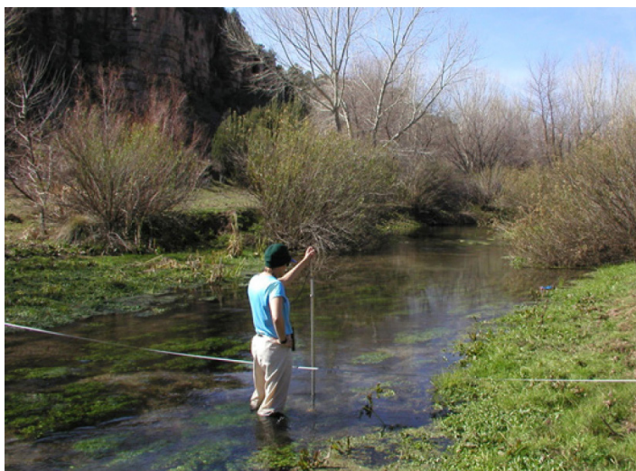
Fig. 46. The channel cross-section with current meter approach is appropriate for discharge measurement in higher volume, wadeable streams.
