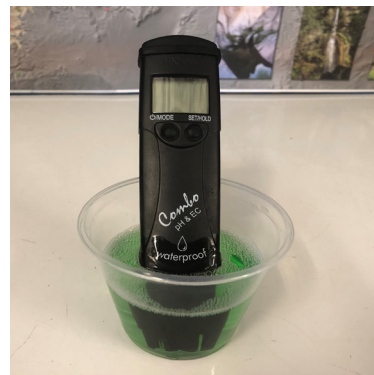
Fig. 53. Water quality probes should be examined after returning from the field and cleaned. Soak them in cleaning solution and rinse thoroughly. Store the probes in an appropriate storage solution.
