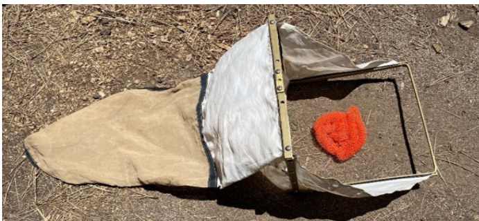
Fig. 28. A Surber Sampler, used for quantitative benthic sampling. The device is placed in-channel with the frame (right) in the upstream direction. The surveyor disturbs the benthos within the frame, and the stream washes the dislodged invertebrates into the net.
