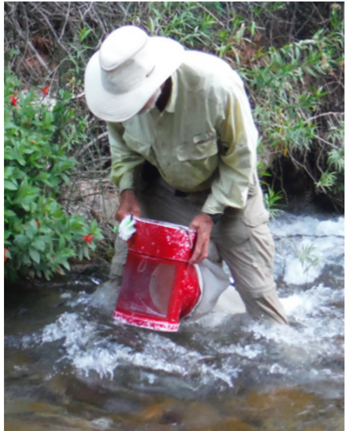
Fig. 29. A Hess basket is used for quantitative benthic sampling of invertebrates in wadeable streams. Hess baskets are designed to collect material as the zoologist disturbs the benthos, while excluding matter in the water column that drifts from upstream.
