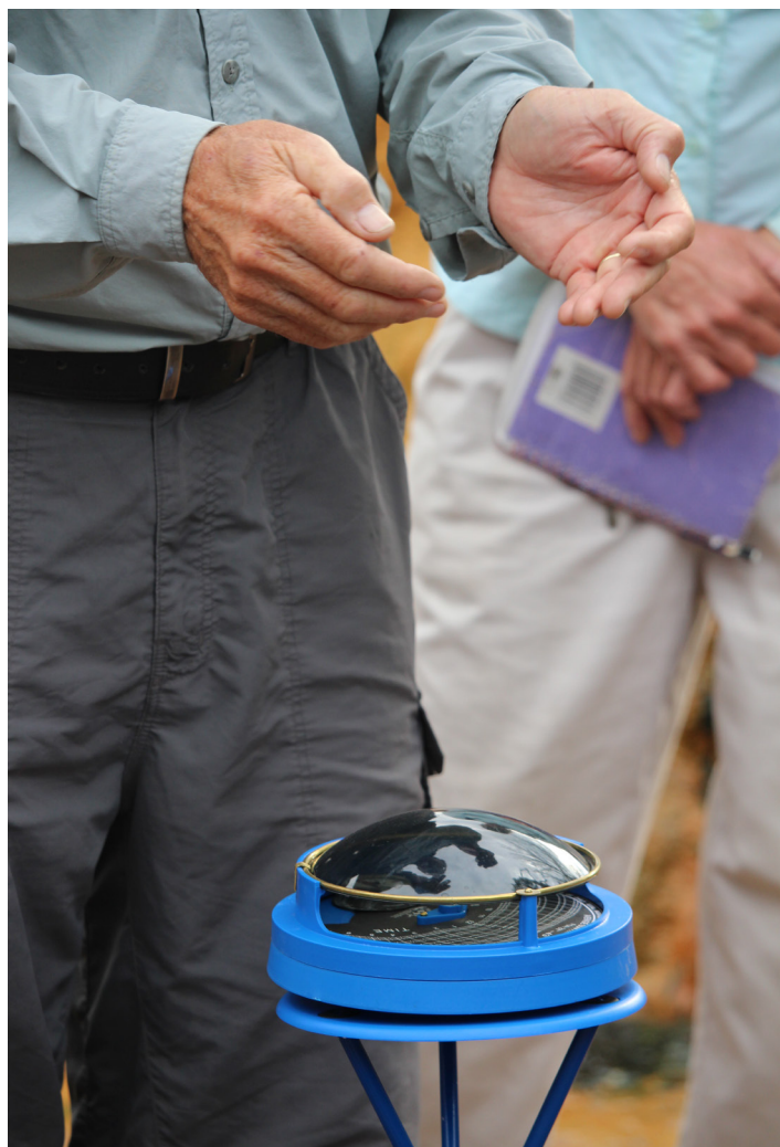
Fig. 39. A Solar Pathfinder is used to estimate monthly photosynthetically active radiation (PAR) at a spring ecosystem.
