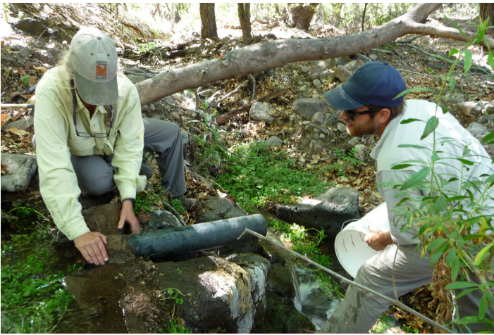
Fig. 40. Surveyors measure spring discharge by creating a dam out of soil or, in this case cow feces, to direct the flow through a pipe. This allows the crew to measure volume captured over time.
