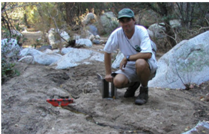
Fig. 44. A surveyor uses a V-notch weir plate (the red device) to measure low volume flows in soft substrate. Note that the surveyor is leaning on a flume, which is not in use.
