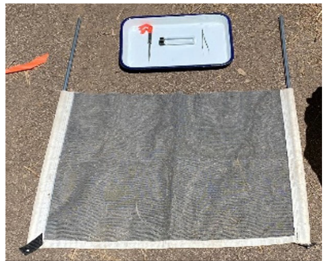
Fig. 27. A kick-net, used for quantitative benthic sampling. This net has an area of one square meter. A smaller net should be used where water depth is less than 50 cm.
