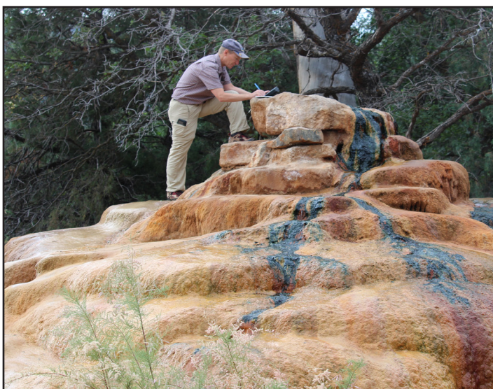
Fig. 13. The GPS coordinate should be recorded as close to the springs source as is feasible. Hydrologist Abe Springer recordings the GPS coordinate on top of the mineral mound formed by a hot spring in La Plata County, Colorado.
