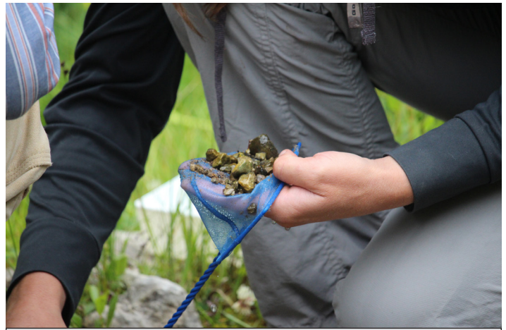
Fig. 31. Coarse substrate materials should be removed from samples in the field to prevent damage to the specimens.
