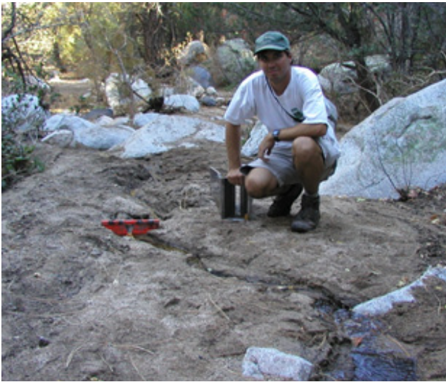
Fig. B.02: Measuring flow using a weir.
