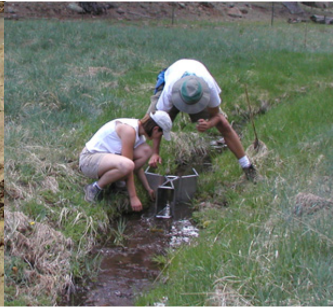
Fig. B.05: Example of a flume used to measure flow.
