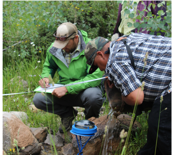
Fig. 2.08: Surveyors record the sunrise and sunset at the source of a spring using a Solar Pathfinder.
