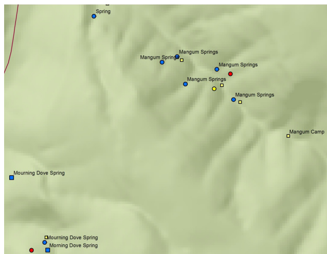
Fig. 2.05: Example of the results of combining several datasets for springs on the North Rim of Grand Canyon. Mourning Dove spring is mapped in four different locations, misspelled in one dataset, and unnamed in two. Clusters of springs, such as in Mangum Canyon increase the difficulty of reconciling datasets.
