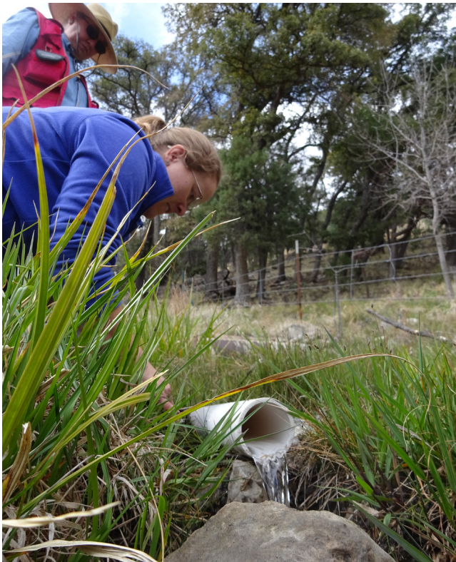
Fig. B.08: Timed volumetric flow capture measurement. SIA photo
