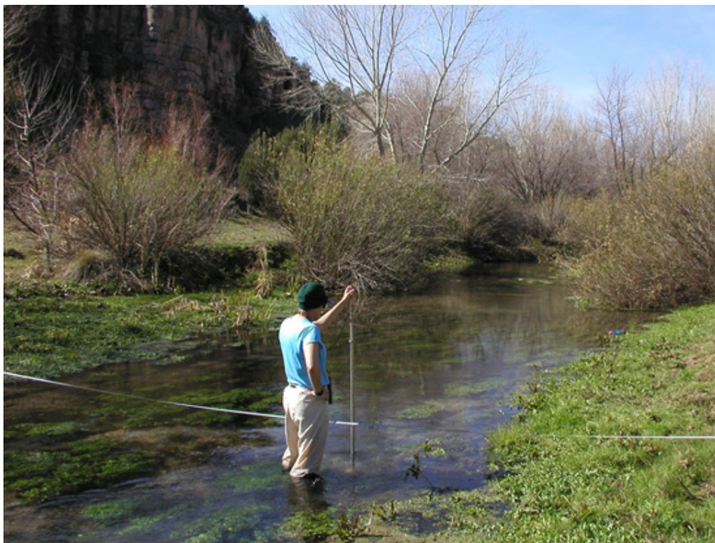
Fig. B.03: The current meter flow measurement procedure.
