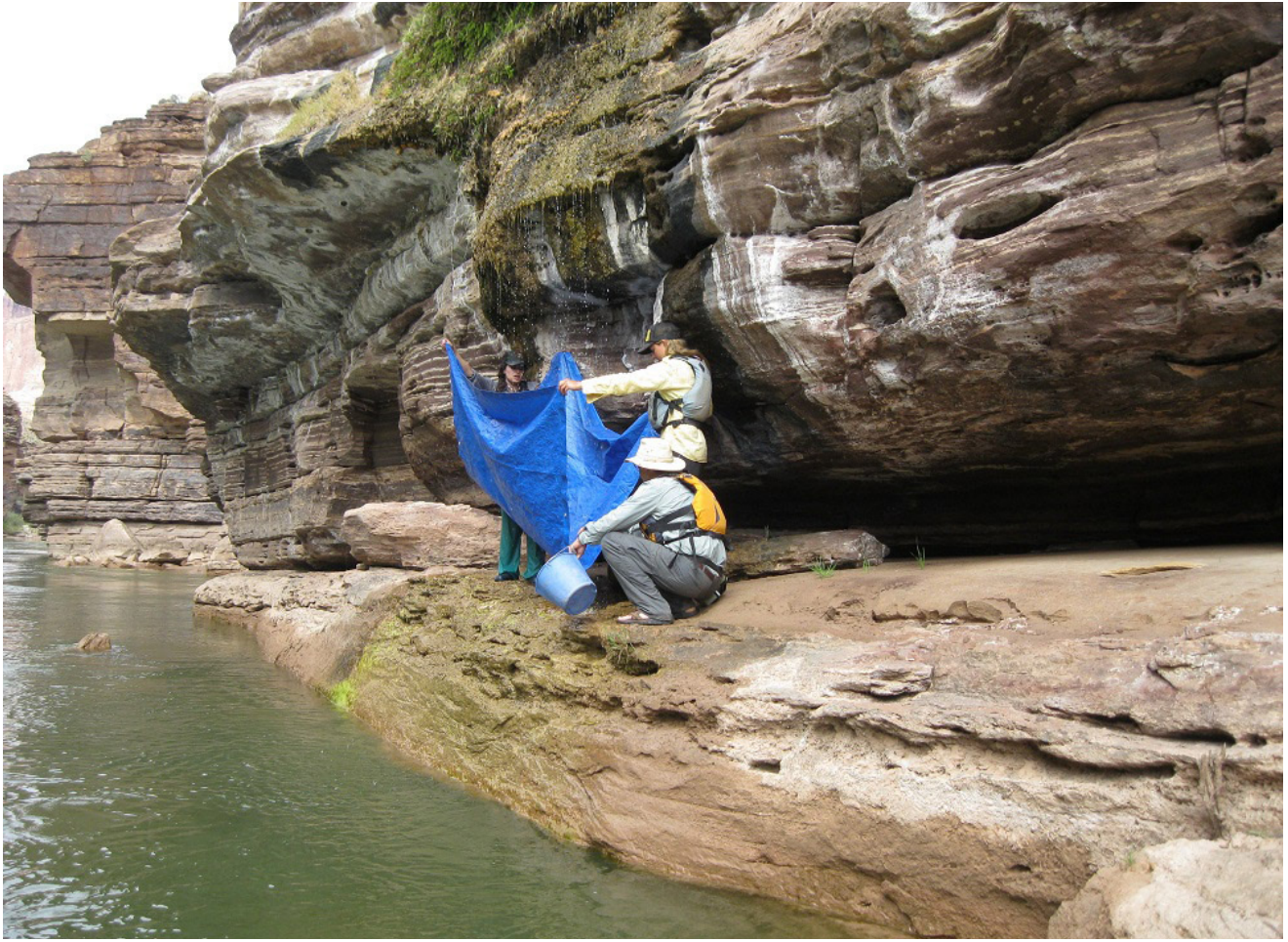
Fig. B.07: Sometimes alternate methods are necessary to measure flow using the timed volumetric flow capture method. At this hanging garden, surveyors captured dripping water using a tarp.
