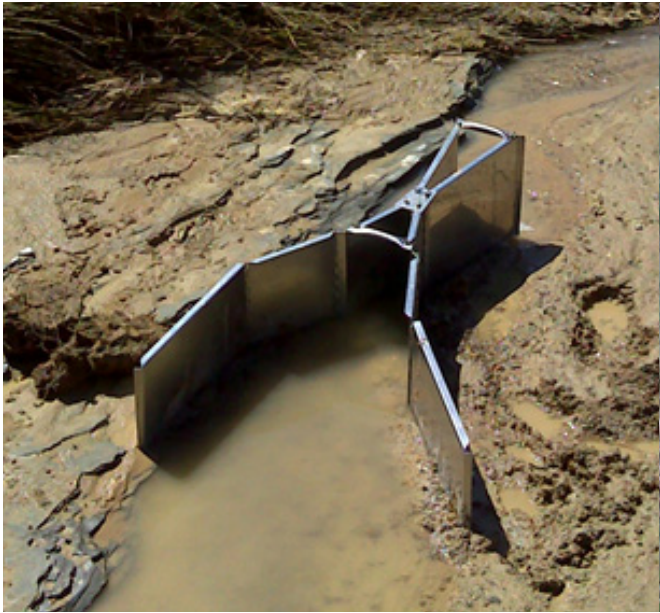
Fig. B.04: A cutthroat flume is installed in a channel.
