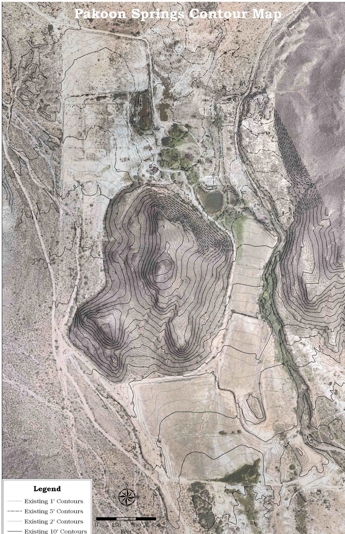
Fig. 6.17: GCWC developed this digitally rectified orthophoto contour map of Pakoon Springs prior to rehabilitation efforts. This provided 1-foot contours with a 90% accuracy, generated from a land survey. The GIS products provided the basis for developing hydrologic, vegetation, and planning maps. Map and analysis completed by Chris Brod.
