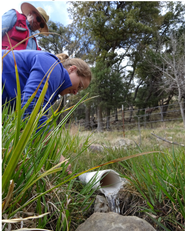
Fig. 2.03: Flow measurements will be affected by plant transpiration during the growing season. SIA photo.
