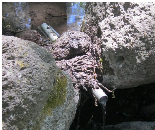
Fig. B.06: Timed volumetric flow capture measurement. SIA photo
