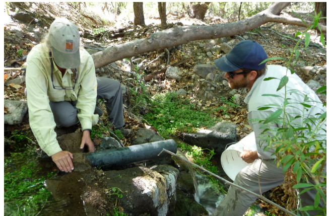
Fig. B.09: Timed volumetric flow capture measurement. SIA photo
