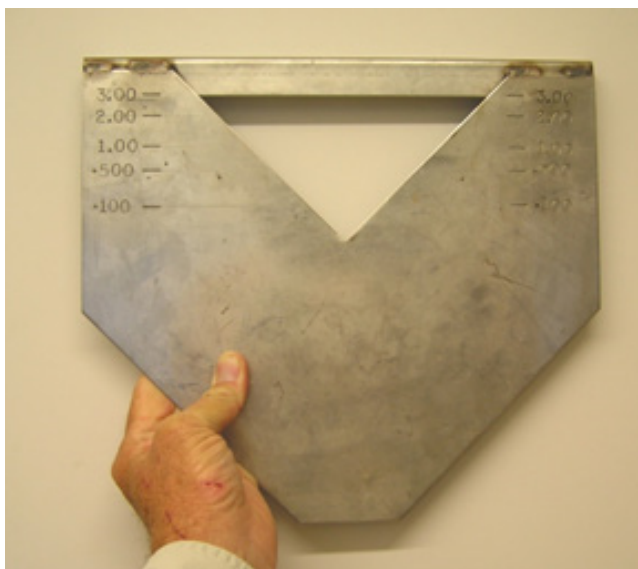
Fig. B.01: Weir plate.
