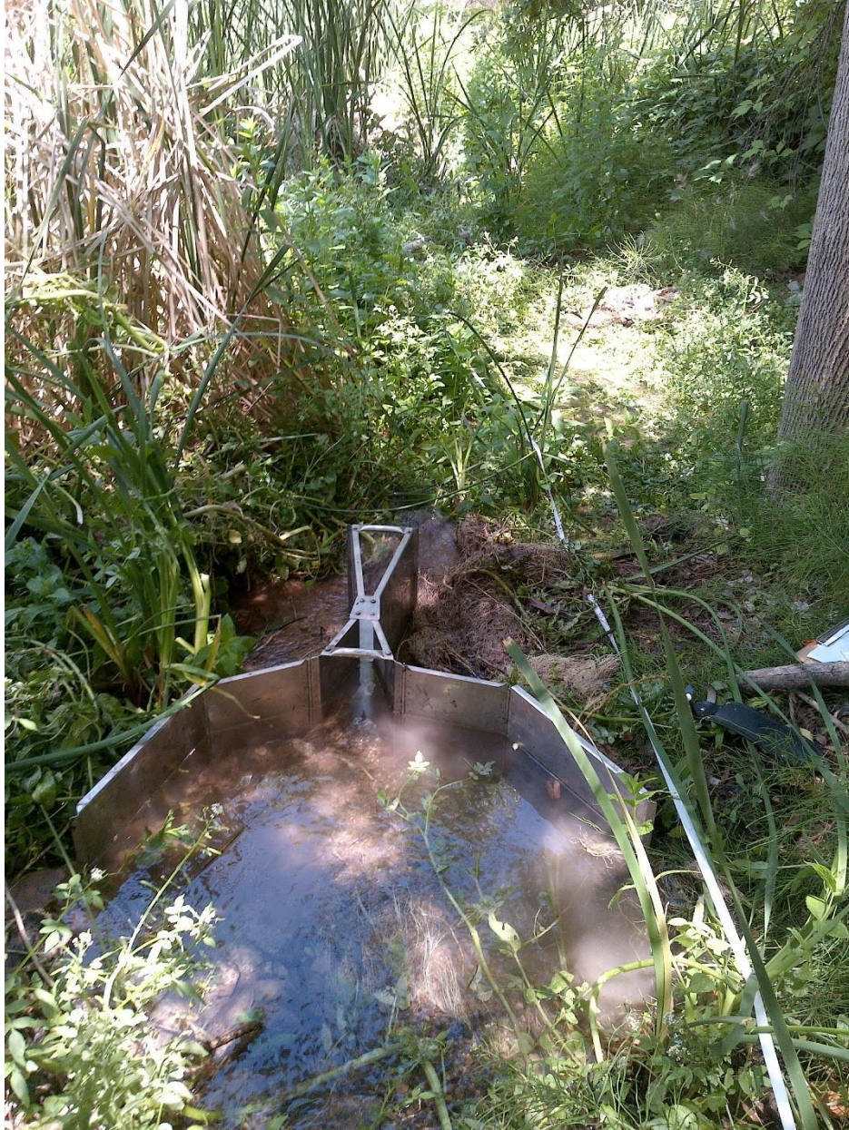
Fig 8.4 Clarkdale Big Spring: Flume placement at second location.
