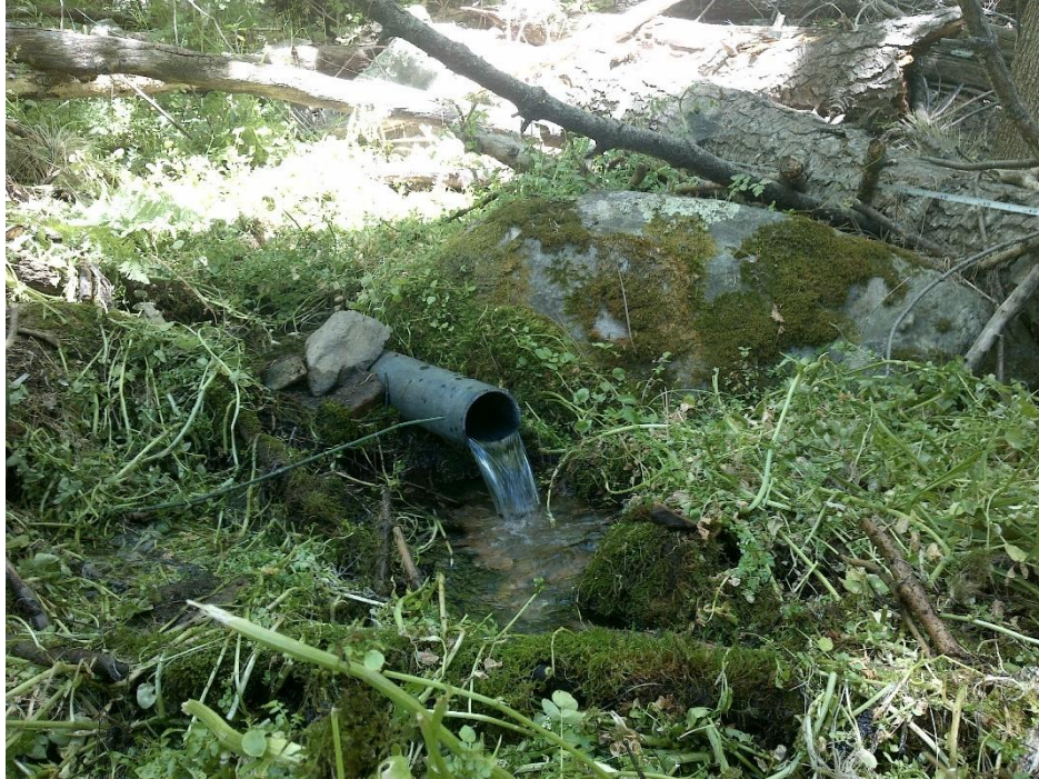
Fig 16.4 Fumann 5 Spring: Surveyors built a pipe dam to measure flow at 22 meters.
