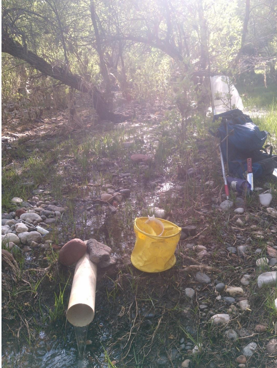
Fig 19.3 King Spring: Surveyors measured flow 150 meters downslope from the source.
