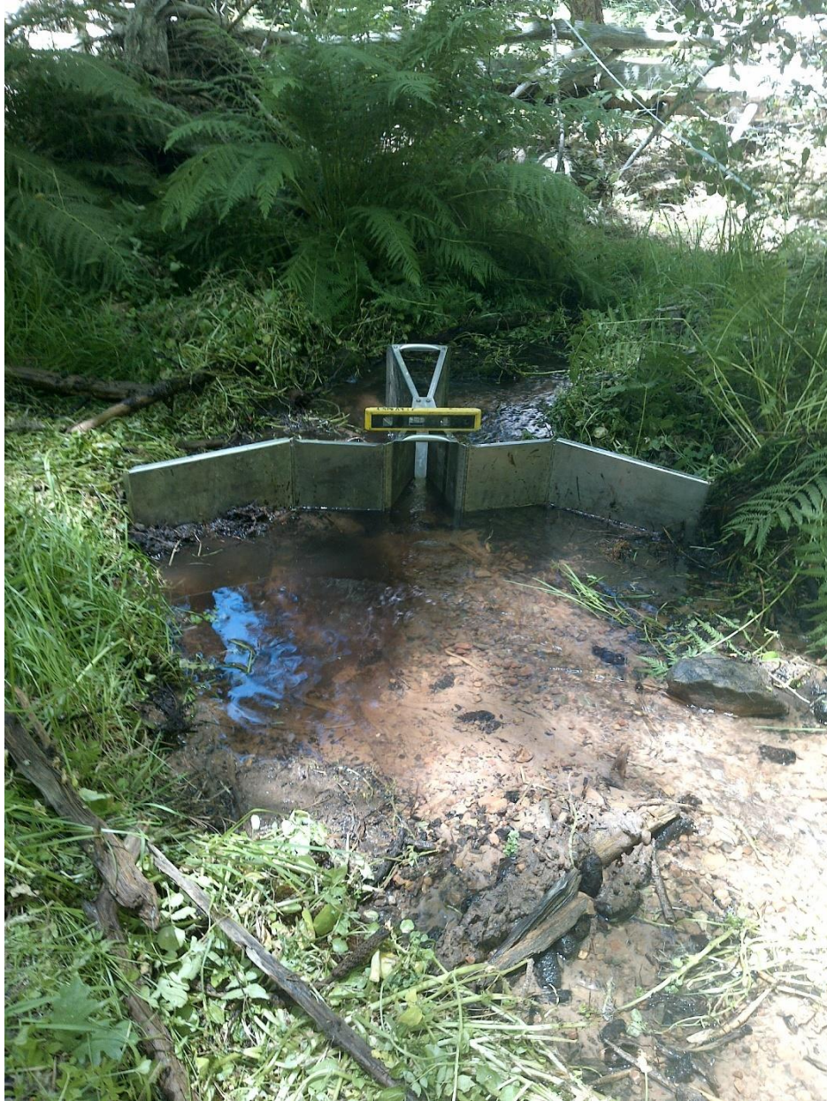
Fig 24.3 Parsnip Spring: Surveyors measured flow with a 4 inch flume at 13.7 meters downstream of the source.
