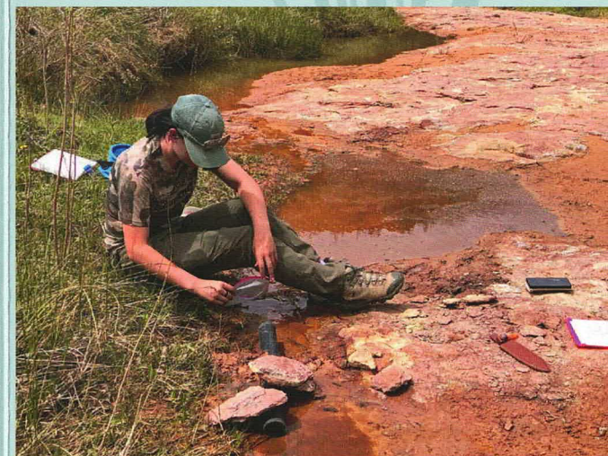
Springs Stewardship Institute crew member measures outflow from a spring.
